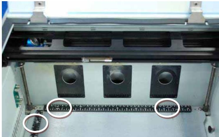
There are three mating pins on the bottom side of the vector grid.
